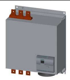
SIRIUS SOFT STARTER, VALUES AT 460V, 50 DEG., STANDARD: 551A, 450HP, INSIDE-DELTA CIRCUIT 3: 954A, 850HP, 200-460V AC, 115V AC, SCREW TERMINALS
